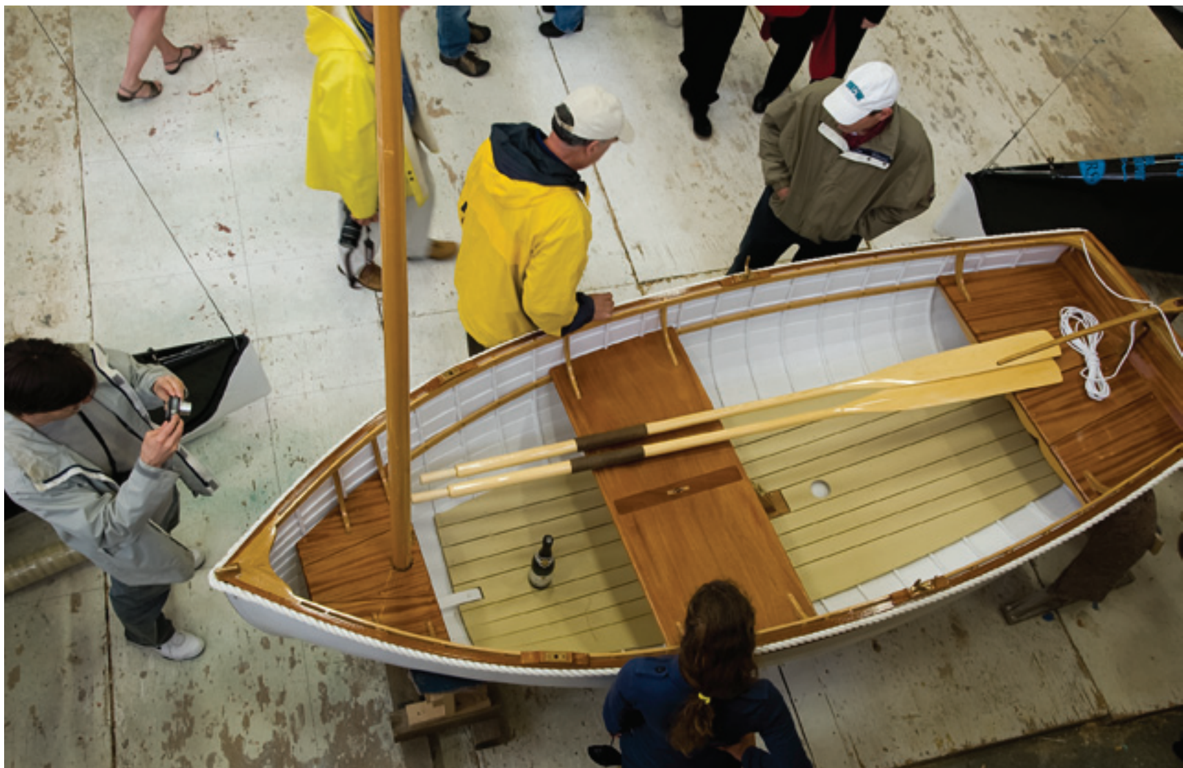
THIS PAGE: STUDENTS AT THE INTERNATIONAL YACHT RESTORATION SCHOOL IN NEWPORT, RHODE ISLAND, BUILT A REPLICA OF DORADE 'S ORIGINAL TENDER, WORKING FROM S&S PLANS AND PHOTOGRAPHS. IT IS LAPSTRAKE PLANKED, USING CEDAR WITH MAHOGANY AS THE SHEER STRAKE, AND IS TRANSPORTED FIXED OVER THE YACHT'S SKYLIGHTS
