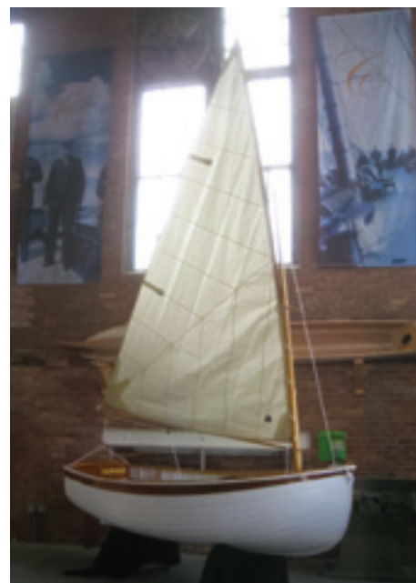
THIS PAGE: STUDENTS AT THE INTERNATIONAL YACHT RESTORATION SCHOOL IN NEWPORT, RHODE ISLAND, BUILT A REPLICA OF DORADE 'S ORIGINAL TENDER, WORKING FROM S&S PLANS AND PHOTOGRAPHS. IT IS LAPSTRAKE PLANKED, USING CEDAR WITH MAHOGANY AS THE SHEER STRAKE, AND IS TRANSPORTED FIXED OVER THE YACHT'S SKYLIGHTS
