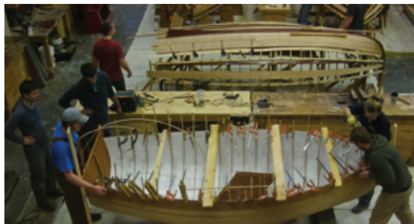
THIS PAGE: STUDENTS AT THE INTERNATIONAL YACHT RESTORATION SCHOOL IN NEWPORT, RHODE ISLAND, BUILT A REPLICA OF DORADE 'S ORIGINAL TENDER, WORKING FROM S&S PLANS AND PHOTOGRAPHS. IT IS LAPSTRAKE PLANKED, USING CEDAR WITH MAHOGANY AS THE SHEER STRAKE, AND IS TRANSPORTED FIXED OVER THE YACHT'S SKYLIGHTS
